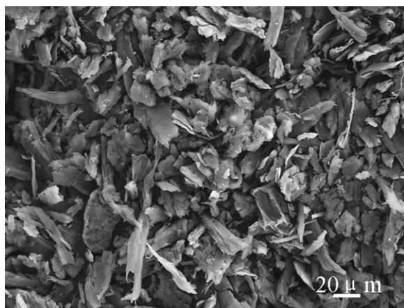
Figure 1 SEM micrograph of a 400-mesh HP sample.
